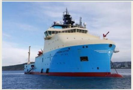
Maersk Supply Service has taken delivery of anchor handling tug supply vessel (AHTS) the Maersk Cutter. The company says that the vessel, delivered on August 5, is the last anchor handling tug supply vessel in a series of two delivered from Asenav in Chile. Maersk notes that like its sister vessel, the Maersk **Clipper**, the new AHTS is able to pull more than 180 tons, and the ample
