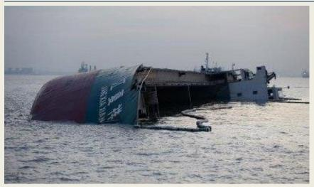
General cargo vessel Jiang Xia Xiang collided tanker Bai Chi at around 0100 LT July 23 Wusong in area, Shanghai, Yangtze river. Jiang Xia Xiang was loaded with 7000 tons of stone, Bai Chi loaded with 30000 tons of crude oil. Jiang Xia Xiang suffered breach or breaches portside with water ingress and danger of sinking. suffered Tanker bow
