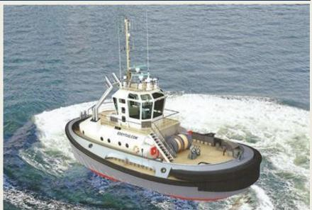
The new model, designated **EDDY 24-70** adopts the same characteristic in-line thruster arrangement as the larger **EDDY 30-65** operating in Bremerhaven. At 24m it is significantly shorter however, with a moulded beam of 11.4m but with a slightly higher bollard pull of 70t compared to the 65t of **EDDY 1**. This arrangement will, according to EDDY Tug "... ensure ease of handling in even the
