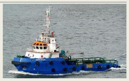
WAF 773 6.44:1 gears to fixed pitch props. Towing gear consists of a double drum tow winch with a capacity for two 750m 48mm wires, gob-eye, tugger, capstan, stern roller, guide pins and shark jaws. Tug was built in 2013 by Yong Choo Kui of Sibu, Malaysia and classed BV R1 +Hull, +Mach,
