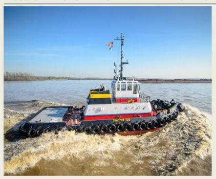
Bisso Towboat Co., Inc., Luling, LA, has signed a contract with the Main Iron Works, LLC, shipyard in Houma, LA, to begin construction of another 4,480 HP ASD Tractor Tug. The new tug, a carbon copy of the recently delivered Becky S.(see earlier story), will measure 100' x 38' x 18.0' and will be powered by two Caterpillar 3516C Tier 3 engines producing main 2,240 HP each at 1600 RPM. Propulsion will be provided by two Rolls-Royce US 205 FP Z-drives featuring 90.4"
