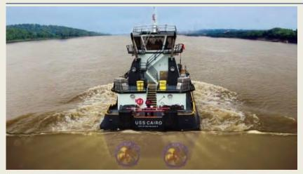
Thrustmaster has been building brown water propulsion equipment for more than 30 years. Now the company's American-made Z-Drive thrusters for inland waterway towboats are the first thruster in the industry to include a built-in mechanical fuse or quick release coupling. The incorporation of a quick release coupling at the input
