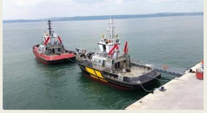
and 14th of this increasingly popular ASD model equipped with Caterpillar engines driving Rolls-Royce Z-drives. Two different customers are involved. Investment at the new shipyard continues alongside a production plan which includes 10 more vessels which, when added to the schedule laid down at Sanmar's existing yard in Tuzla, will bring the company's production for the year to 25. On the picture is seen the **Bogacay 12** and **Bogacay 13** (*Press Release*)
