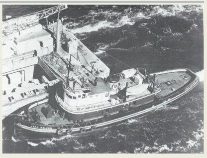
line holds the tug tightly alongside the barge and controls turns to the barge's side. *(Source: On the Hawser by Steven Lang and Peter H. Spectre)*
