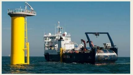
CT Offshore installed the first inter-array cable at Dong Energy's Gode Wind 1 + 2 offshore sites yesterday. Crew on board cable laying vessel (CLV) **SIA** had been prepared since Thursday, waiting for good weather conditions to install the J01-I02 cable. The company is using its new trencher ROV, the CTO 107-1100, which has an operating
