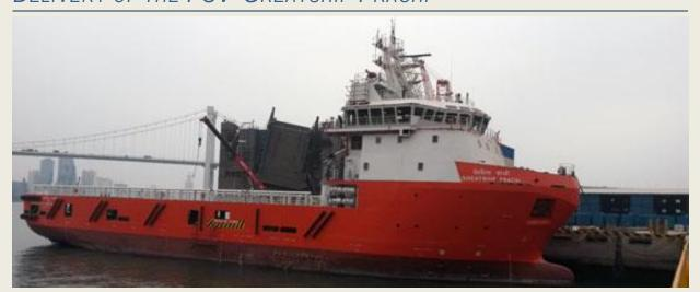
Greatship has taken delivery of the 'Greatship Prachi', a 4,000DWT platform supply vessel constructed at the Xiamen Shipyard in China by Nam Cheong this year. 'Greatship Prachi' is a DP2 vessel, with accommodation for 56 persons and is compliant with the SPS code 2008. The vessel is 78.0 metres long, has a beam of 18.60 metres and a draught of 6.0 metres. 'Greatship Prachi' has now
