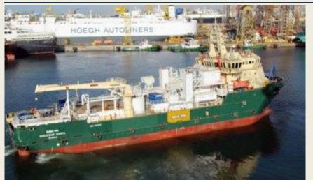
Classification society **IRClass** has recently completed the survey and certification of 'Greatship Ramya' during conversion from an offshore supply vessel to a well stimulation vessel for Schlumberger under its class. single Well stimulation vessels are one of the most critical ship types in the
