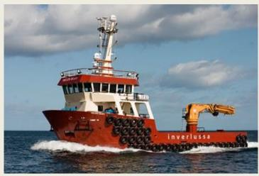
the operational requirements of the job. **Helen Mary** is a valuable addition to Inverlussa's expanding fleet. She has a length o.a. of 27.30 mtrs a beam 10.00 mtrs a draught of 2.75 mtrs and a depth of 3.50 mtrs. The three Caterpillar C18 develops a total output of 1,800 bhp @ 1,800 rpm.She has a bollard pull of 25 tons and a free sailing sspeed of 12 knots and is classed Bureau Veritas. *(Press Release Macduff)*
