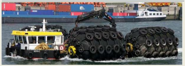
Mariflex **Kevin C** was seen enroute Dolphins 90-91 in Rotterdam Maasvlakte basin 2 with 4 large pneumatic Rubber Fenders designed and fabricated by BARU for the STS operation between the *Leonid Loza* (274 mtr, 156630 DWT) and the *Hamilton Spirit* (274.48mtr, 158.099 DWt)(Photo's: Gerrit Jan Postma – www.aerolin.nl (c)
