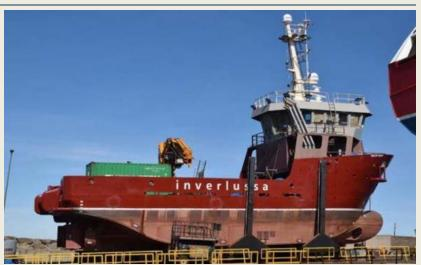
system, and a 50 tonne towing anchor handling winch. Main engines are 3X600 Caterpillar C18s total power is 1800. Triple screws fixed pitch 1400mm props in nozzles with high lift rudders. *(Photo's: Iain Forsyth)*
