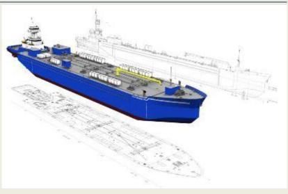
ABCU, Oceans Towing Vessel Unlimited Service certified under SOLAS/IMO/MARPOL. *Gult Carrier ATB Double Hull Oil Barge:* Dimensions: 399'x 74'x 30'; Capacity: 80,000 BBL; Bow Thruster: (1) Thrustmaster retractable azimuthing thruster, 750HP; Main Generators: (2) John Deere 99kW; Classification: ABS [IA1, Unlimited Oceans, Permissively Manned. *(Press Release)*
