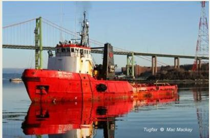
Beaufort Sea offshore oil, and the tug/supplier was one of several built to work in the western arctic area. It is powered by a pair of GM engines totalling 7200 bhp, giving it a bollard pull of 90 tonnes, and is purpose built for harsh weather. When Dome got in to financial trouble the company was sold to Amoco Canada in 1987. However oil work in the Beaufort came to an end and in 1995 the
