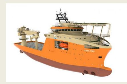
depth capability of 3,000 metres single fall, and an auxiliary crane with a capacity of 25 tonne and a single fall depth capability of 2000 metres. There will be a working deck area of 1,100m2 and а large working moon-pool of 7.20 x 7.20 metres. With a minimum deck strength of 10t/m2 and specific areas strengthened to take 25t/m2, carriage and deployment of equipment heavy and
