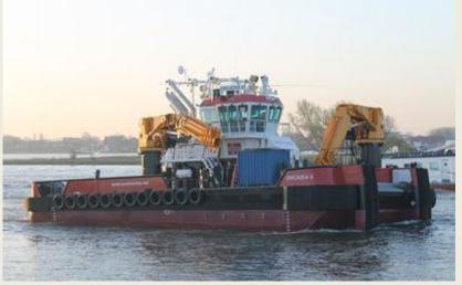
Last week was seen the Damen built yard number 571683 MultiCat 2613 Orcadia II (Imo 976643) being transferred to the Damen Hardinxveld yard for outfitting. The Multicat is on order for Scot Marine and is the second for this owner. The standard dimensions for this type of vessel are Length (meter)26.25; Beam (m) 13; Power (BKW)2850; total Bollard pull max (tonnes)45 and a Crane capacity (tm)15.
