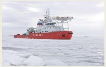
On April 2, 2015, innovative multipurpose icebreaking emergency and rescue vessel Baltika successfully completed her ice trials, says Sea Rescue Service of Rosmorrechflot. The tests were held in the Kara Sea off island Bely near the Ob Bay and at port Sabetta. The tests included the assessment of the ship controllability and maneuverability conditions, measuring of the hull
