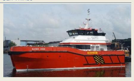
kW. The vessel is specifically designed for working further offshore with a fuel capacity of 29,000 litres and fresh water capacity of 2,900 litres. The vessel achieved a speed of in excess of 27 knots
