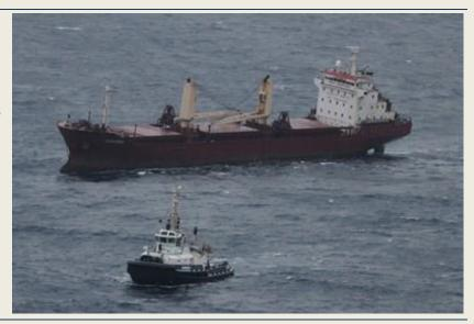
design RA3200.W tug has a length of 32.00 mtrs a beam of 12.00 mtrs and a draft of 5.80 mtrs. The two ABC type 12DZC diesel engines develops a total output of 7,200 bhp which results in a free sailing speed of 13.5 knots and a bollard pull of 83 tons. The tug has a grt of 487 tons a dwt of 186 tons and is classed Germanischer Lloyd. (*Photo: Capt. Lawrence Dalli - www.maltashipphotos.com*)
