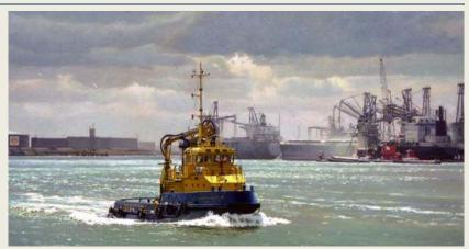
Damen shipyards- Gorinchem built vessel has a length of 29.71 mtrs a beam of 7.2 mtrs and a raft of 2.90 mtrs. The two Catepillar 3412 E TA/ engines develops an total output of 97 kW. View painters website <a href="https://www.nicompeeters.nl">www.nicompeeters.nl</a>
