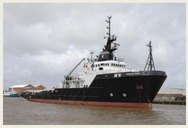
as relief ETV on the occasions when the regular vessels were undergoing refits. The 12,000bhp, 135 tonne bollard pull vessel is powered by two MAK 8M35 diesels driving twin controllable pitch propellers and as with the other ex Klyne tug has received the Resolve prefix to its name to become **Resolve Earl**. (Source: Maritime Journal; Photo: Paul Gowen)
