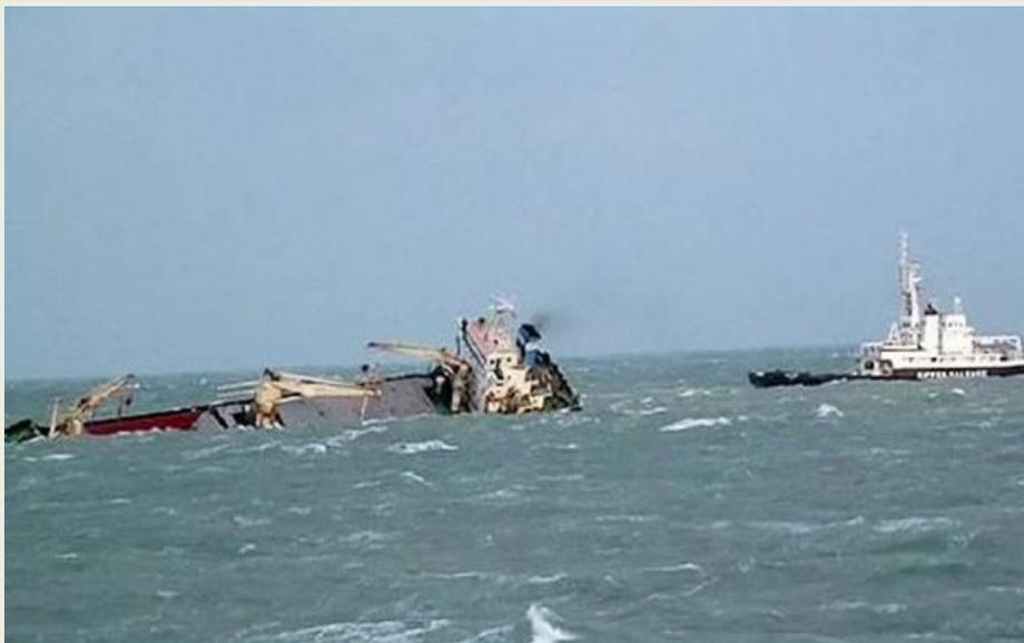
General cargo vessel *Eastern Amber* capsized some 25 nm northwest of Jeju Island, South Korea, East China sea, on Mar 11, while being towed by a Japanese salvage tug **Koyo Maru** to Busan, after vessel was breached in a collision off Gunsan. Freighter was loaded with timber, at the time of an accident there were no crew on board.
