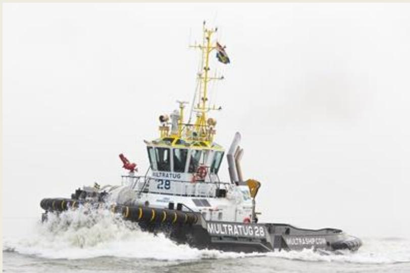
LEADING towage and salvage specialist Multraship has welcomed **Multratug 28**, an energy-efficient hybrid Damen ASD 2810-type tug with state-of-the-art FiFi 1 firefighting capabilities, into its fleet. Damen’s ASD 2810 Hybrid is a new design and this is the second of its class to be built. It features diesel-direct, diesel-electric and battery-powered propulsion systems. This hybrid configuration will enable
