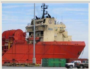
The anchor handling tug supply vessel (AHTS) **Edison Chouest** has arrived today in Port Fourchon after being towed by the AHTS **Gulf Champion** from Trinidad. An anonymous source tells gCaptain a fuel return line failed on the vessel's port main engine, a CAT 3616. The resultant fire burned up the engine and both winch engines and wiring on the deck above, in addition to causing a stack fire. (Source: gCaptain)
