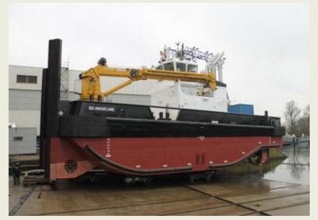
Last week was seen at the Damen Shipyard Gorinchem: Netherlands the launching of the SD **Angeline** (Imo 9648544) a Multicat 2613S with yard number 571681. The vessel is under construction for Serco Denholm. She has a length of 26.25 mtrs a beam of 13.00 mtrs. Her total power output is 2,850 kW with a bollard pull of 45 tons. The crane has a capacity of 15 tm. The Multicat is a proven design
