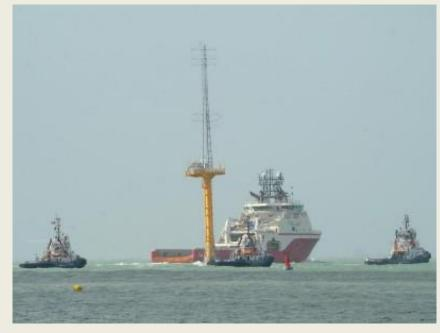
**Bison**, an offshore Boa support vessel, has just completed her work at the Fecamp offshore wind farm. During the installation of a met mast at the Fecamp offshore site, the vessel was in charge of the pre-lay of anchors for a gravity base structure and ROV work during submerging. Supplementing the data collected since 2007 in technical and environmental studies, the met mast will seek to determine the speed and direction of wind,
