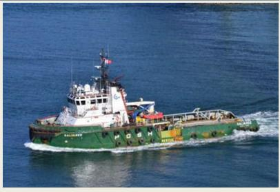
mtrs and a draught of 4.80 mtrs. She was built by president Marine Pte. Ltd. Shipyard – Singapore under number 303. The two Wartsila main engines develops a total output of 2,970 kW (4,036 hp) and a free sailing speed of 13.3 knots. She has a grt of 874 tons a dwt of 838 tons and is classed Bureau Veritas I  $\clubsuit$  Hull  $\clubsuit$ Mach. Tug-Supply Vessel Unrestricted Navigation. *(Photo: Robert Etchell)*
