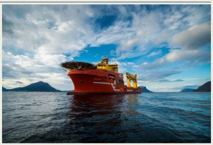
into contract with Technip\_for the supply of OCV. The vessel will be equipped with Reach ROVs and manned by Eidesvik marine personnel and Reach ROV personnel and engineers. The vessel has a length of 145 m and a beam of 31 m. It is equipped with 2 offshore cranes on 400T and 100T respectively and a Carousel with a capsity of 4400T flexible pipes. The vessel has classification ICE 1B which means it is prepared for operation in arctic waters. (Source: Offshore Energy Today)
