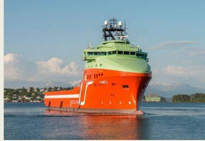
long, 20 m in width and with accommodation for 24 persons. Salt 100 combines innovation in design and technology to improve operating costs, improve safety and secure more efficient operations. Fuel consumption is low, and the vessel was the first of its kind to incorporate a new and more efficient cargo handling solution. The vessel is under a two-year contract with Statoil with two additional one-year options. *(Source: Offshore Energy Today)*
