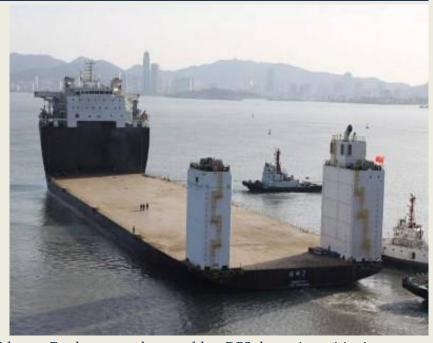
meters and design speed of 13.5 knots. Furthermore, the vessel has DP2 dynamic positioning system and unmanned engine room and all moving tail buoyancy tank. (Source: Offshore Energy Today)
