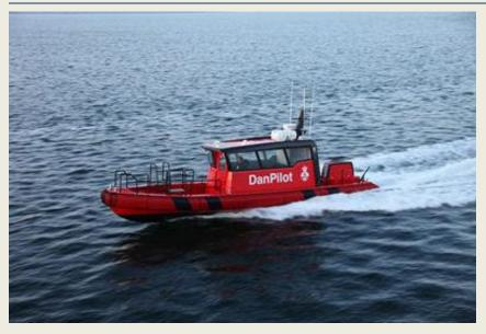
Tuco Marine delivers the first vessel specially designed and equipped for Pilot services to the shipping company Sea Charter A/S. The vessel, which has been built at Tuco's facilities in Faaborg, is an ProZero 12m DC. During this week it has been sea trialed in the cold January conditions offered by the bay off Faaborg. The ProZero 12m DC features, a complete protective cabin for the crew. So the tests could be carried
