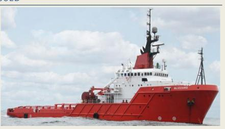
two MaK 8M35 diesel main engines develops a total output of 12,000 hp. Her free sailing max. speed is 14 knots and bollard pull 144 tons. Her grt is 2,311 tons and nrt is 693 tons. It is likely that she will renamed **Resolve Blizzard**? The **Blizzard** is the former **Maersk Leader**. (*Photo: Resolve*)
