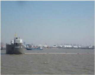
forward 17 mtrs also. She has a grounding draft of 20 mtrs. *Cargo capacity:* Deadweight 21.000ton; Deck area 4500m2; Free deck length 120m; Deck load 20ton/m2. Ballast system type Diesel-electric pumps with a capacity of 6,400 m3/h (4 x 1,600 m3/h). The two main generators develops a total output of 840 kW. The auxiliary generator delivers 60 kW. The barge is classed Lloyds Register of Shipping +100 A1 Pontoon, Submersible to a maximum draught of 17m, IWS, *(Source: Bram de Feijter)*
