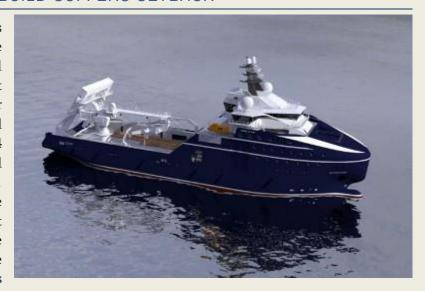
set for the Q1 2017. According to Rem Offshore, the remaining terms are unchanged. The building cost for the vessel is approximately NOK 800 million (\$133.3). The vessel is of the **Vard 2 06 design** with overall length of 100 meters and a beam of 25 meters. It will be equipped with a 150 ton offshore crane, ROV hangar, prepared for A-frame and accommodation for 90 people. Rem Offshore recently received notice of contract termination for two of its platform supply vessels chartered for
