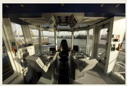
possibility onboard viewing tomorrow's tugboat. Together with Newbuild captains all the different ideas were put on paper and were later on put into a 3D model to see how this would improve operation of the tugboat. Alphatron's bridge design, called Alphabridge, was able to comply to this new market demand because of its modularity. This ergonomic design is based upon 2 approved screens, showing RADAR and ECDIS at the fore
