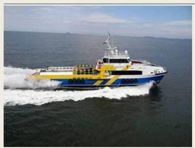
BS Camburi, a 36-meter Monohull Crewboat built in Brazil by Engenharia Arpoador the Petrobras type P2 specification has launched and delivered. Designed by Incat Crowther, the (36-meter) aluminum 118-foot crewboat is powered by triple CAT C32 ACERT diesel engines coupled to three Thrustmaster DOEN DJ290 waterjets. Designed to Petrobras type P2 crew boat spec, this vessel will transport up to 70 passengers and crew as well as carry 50 tons of deck cargo plus fuel and fresh water
