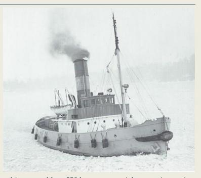
The **Simson**, which was built in 1915 and is powered by a 550 horsepower, triple expansion engine, was probably used for coastal work in her early days. Today, with her modest horsepower, she does
