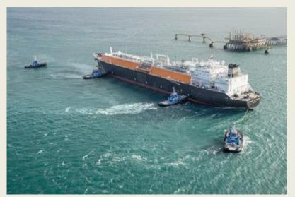
Lamnalco team provides towage and marine support services for LNG carriers with four 70 tonnes bollard pull 32m ASD tugs. (Press Release Smit-Lamnalco)
