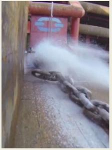
controlled and predictable manner. Activation of the ControlCutter will ensure the chain or wire is cut instantly without any damage to either the winch system, deck equipment or vessel in general. Operations can again proceed after the chain or wire has been retrieved from the seabed.
