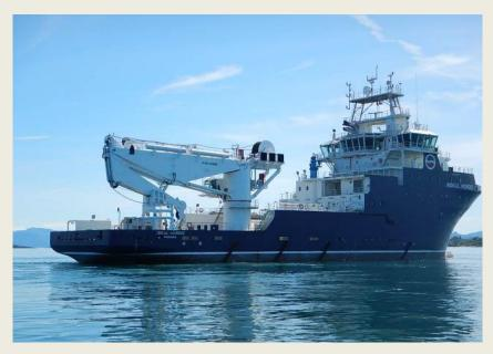
installed with a WROV and all ready for the new project," said **K**jell Gauksheim, Executive Director of Nordic Maritime. **Nordic Prince** is a DP2 VS470 MKIII subsea service vessel capable of ROV / IMR operations. It is specially customised and equipped to perform IMR/ROV work. The vessel has a 100-tonne active heave compensated offshore knuckle-boom crane built-in and swell compensation systems
