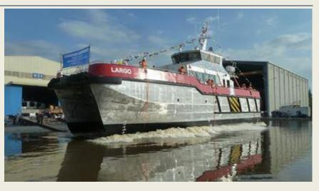
increased range and wind turbine supply; - water jet propulsion offering a 27.5 knots top speed; - equipment and comfort inspired by business class standards; - carefully designed wheelhouse ergonomics. *Main characteristics* Length: 27.40 m; Beam: 8.00 m; Maximum draught: 1.30 m; Maximum speed: 27.5 kn; Propulsion: 2 waterjets; Hull / superstructure: aluminium; Crew: 3 p.; Industrial personnel: 12 p.; Cargo capacity: 10 t; 3 containers 10' *(Press Release Piriou)*
