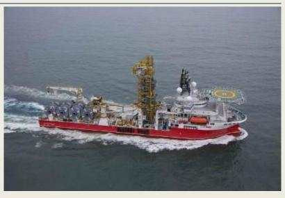
capacity of 550 tons, the vessel will be employed mainly to install umbilical and flexible flowlines and risers to connect subsea wells to floating production units. According to Technip, these installations will take place in waters up to 2,500 meters deep offshore Brazil, including in the presalt area. (Source: Offshore Energy Today)
