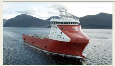
World's largest LNG powered PSV enters Statoil chart. Rem Eir, build no 356 from Kleven Verft, was delivered to Remøy Shipping November 26, 2014. With a length of 92.5 metres and a deck capacity of 1080 m2, Rem Eir is the world's largest environmentally friendly LNG powered
