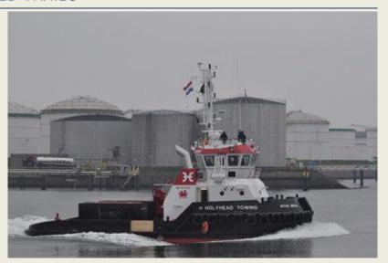
that during the trails the tug will reach a bollard pull of 30 tons and a speed of 10 knots. *(Photo: Ruud Zegwaard)*
