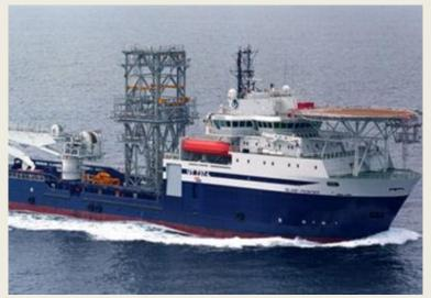
platform. Sleipner Øst is a gascondensate field in the central North Sea. The field has been developed using an integrated processing, drilling and accommodation platform with a gravity base and associated subsea structure templates. Island Frontier is a riserless well intervention vessel that provides access to the subsea well through a Well Control Package. Island Frontier was built at Søviknes Verft AS in 2004. It is 106 metres long, with a beam of 21 metres. The
