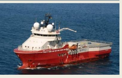
EMGS. The survey will be done using the vessel **BOA Thalassa** and is expected to start directly after the ongoing survey in Malaysia is completed. **BOA Thalassa** is a purpose-built 3D EM vessel with the capacity to carry 200 receivers. It is equipped with parallel source systems, including winches, cranes and hydraulic feeds. *(Press Release)*
