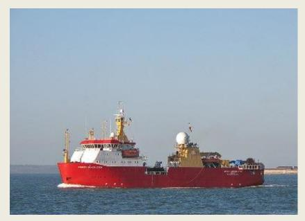
DPII charter vessel **"RRS** Ernest Shackleton" undertook the offshore element of the project. Among the company's most significant charters, the **RRS Ernest Shackleton** is an 80m. DP2 multi-purpose survey vessel accommodating up to 48 survey personnel for duration of excess of 50 days. The vessel is ideally suited to the more exposed offshore sites and can operate comfortably in 2m significant wave height. Osiris Projects Commercial Manager Patrick
