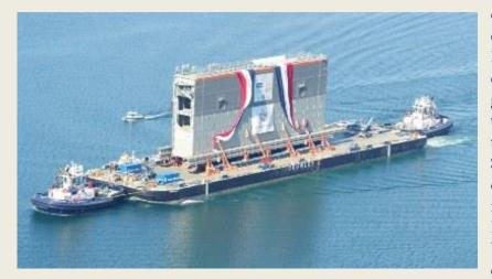
4 was capacity. The **455** contracted by Sarens, а Belgium-based heavy lift company, to transport the gates from Cristóbal, a port on the Atlantic side of the Canal, to Grupo Unidos por el Canal, SA's (GUPC SA) construction dock, which was built to receive the gates on the canal's Pacific side. The 105-foot wide barge, currently the largest capable of transiting the Canal,
