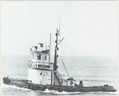
accommodations – the **Lower T** has room only for a galley and a head under the wheelhouse. A distinct advantage is the good visibility that this design affords the pilot. The stack is quite narrow and runs high up the mast to discharge the engine exhaust. This photograph shows some of the essential elements of a modern harbour tug – the air horns and radar on the wheelhouse roof and the VHF antenna and towing lights on the mast. (Source: On the Hawser by Steven Lang & Peter H. Spectre)
