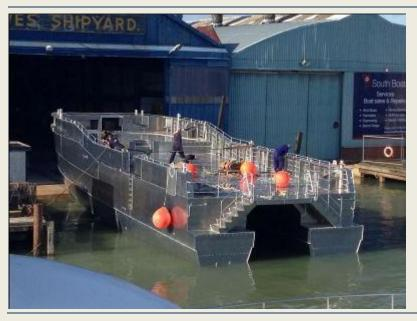
Last week was seen Iceni Venture being hauled out on the 27th October, for outfit. She is the first South Catamaran 22 mtrs built by South Boats IOW Designers and builders of offshore wind farm crew transfer vessels and commercially operated catamarans. The vessel has a length of 22.80 mtrs a beam of 7.73 mtrs and a depth of 3.91 mtrs with a displacement of 53 tons. She will be classed DNV № 1A1 HSLC R1 Windfarm Service 1 (Source: South Boats)
