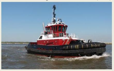
Horsepower: 5,150 HP @ 1,600 RPM Main Engines: (2) Caterpillar 3516C (B Tier 3 marine rating) propulsion diesel engines. Propulsion: (2)Schottel Model SRP 1215FP in Nozzles Z-Drives. Main Generators: (2) John Deere 4045AFM85 Tier 3, 99kW 480V @ 1800RPM marine diesel generator Hawser Winch: (1) Markey Machinery Fairleader 50HP
