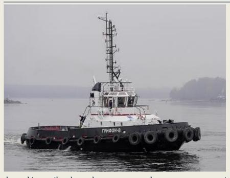
The tugboat **Griphon-8** of the project 90600, building No 944 has been delivered to the Customer, the Tug Company "Griphon" Ltd. At this point all required arrangements has been held for its passage to area of operation. The tugboat is intended for towing and berthing operations roadstead's harbor. coastal areas which comply with R3 navigation area, refloating of ships and firefighting operations at floating and
