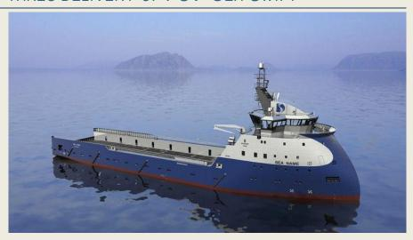
1000m2 deck area, clean design, diesel electric propulsion and the X-bow design which significantly reduces fuel consumption. Following the delivery of 'Sea Swift', Deep Sea Supply has 15 AHTS vessels and 25 PSVs in operation, in total 40 vessels. (*Press Release*)
