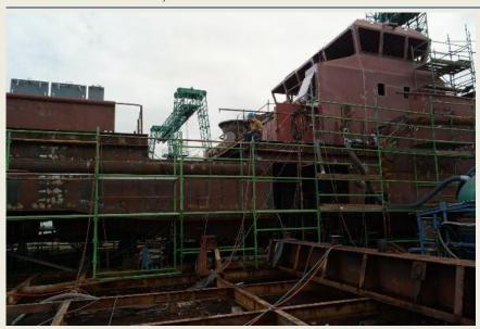
Since the last update of **Barney** a lot has changed again. With the current the situation is now, the hull would be nice on schedule to be ready for transport. Push fender sitting all together including the bow thruster, and push fender is already attached to the hull. Accommodation is on the hull, and it has also been completely welded and has already been painted since last Monday 6-10-2014
