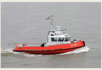
develops a total output of 894 bkW (1,216 bhp). She achieved 16.1 ton bollard pull. Her speed is 11.3 knots The tug is classed Bureau Veritas I X Hull • MACH TUG Coastal Area incl. tonnage certificate (Source: Damen)
