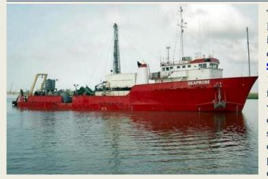
The National Transportation Safety Board (NTSB) issued the report of its investigation of the sinking of the oceanographic research vessel **Seaprobe** in the Gulf of Mexico on Jan. 18, 2013. The probable cause of the flooding and subsequent sinking of the vessel was the decision of the owner to delay making permanent repairs to the starboard-side exhaust trunk and covering six of the vessel's freeing ports, leaving the vessel susceptible to down flooding from boarding seas.
