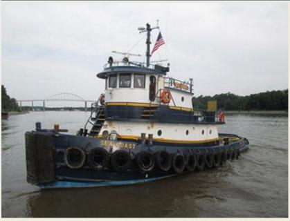
Dann Marine Towing, LC., is a fifth generation family owned and operated tugboat company based in Chesapeake City, MD. The model-bow twinscrew tug Sea Coast was built at Rayco Shipbuilders in 1980 and is one of Dann Marine's 18-tug fleet. She is 65 feet overall with a 24-foot beam and an 8.9-foot draft. carries 16,000 gallon fuel and 5,000 gallons of water. One of many versatile tugs working in US waters of this class, she is registered for Coastwide
