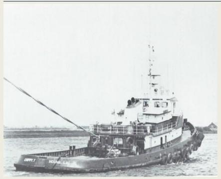
The **Chippy T.**, one of the first generation offshore oil tugs built especially for the business, towing a drill rig. She was built in 1970 at Slidell, Louisiana, and is 150 feet long overall, with a formidable 5600 horsepower rating. After the onset of offshore oil drilling in the Gulf of Mexico, conventional tugboats were used to serve drilling rigs, but hard experience dictated that a new class of tug was required. The United States the world became leader in the design and
