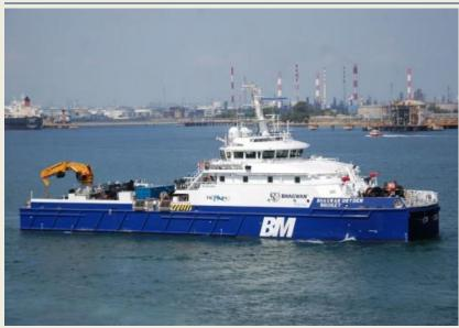
announced to the ASX on 28 August 2012, the Bhagwan Dryden is a state-of-the-art 57 metre DP2 hybrid catamaran, with Neptune-supplied permanent air diving, and survey inspection capabilities. The vessel has the capability to work in shallow waters, offering operational efficiencies at these depths and is also fitted with a TMS light work class Comanche ROV. The Bhagwan Dryden will be based in Australia working
