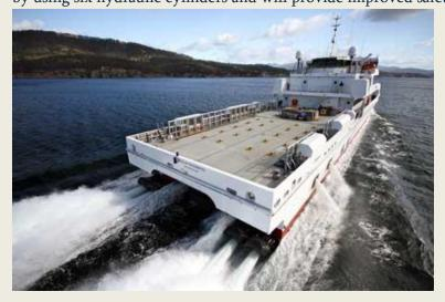
up to Sea State Four. The vessel can also operate in 40-knot winds and seas of up to three metres. Incat Tasmania said the vessel's anticipated design speed was 36 knots with a service speed of 30 knots. On the first day on the water, the vessel achieved a speed of 38.7 knots lightship. She is powered by four 2,880kW engines coupled Hamilton waterjets. Designed in Australia, the vessel's 16-metre beam was determined by the width of the Volga-Don Canal that it must transit
