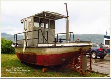
grapple anchor and warping machine (winch). Setting out the anchor, the tug then connected to a log boom and winched itself up to the anchor. The gearing of the warping winch allowed them to pull far more than they could on their own engine and prop. They were also able to warp themselves portaging over land. between lakes, often on winter ice or snow roads. Using their heavily guarded working in props they
