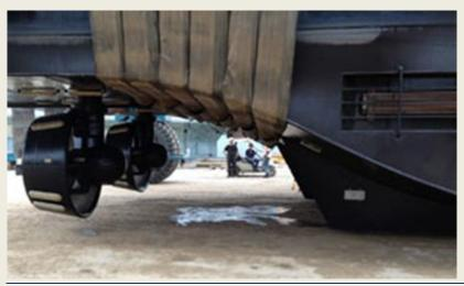
American Way went to work for ACL in the Baton Rouge, La., barge fleet, while the 75-foot American Spirit is headed for the Gulf Intracoastal Waterway between New Orleans and Houston. Z-drives, which provide a 360° directional option, are more efficient than a traditional rudder configuration because they focus all of the engine's force toward pushing the boat in the direction the
