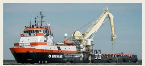
were installed using the HOS Mystique without any incident, on schedule and within budget." The Jones Act compliant 250 ft (76.2 m) offshore construction vessel has accommodations for 62 personnel, a 70 MT AHC crane with 2500m wire,
