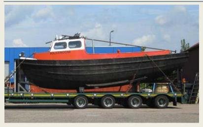
was loaded on a truck by van de Vlist transport Transport Group. On day later on the 22nd August the boat arrived in Genua and was unloaded and direct operational. The 1968 built workboat has a length of 9.08 mtrs and a beam of 2.73 mtrs and a depth of 1.50 mtrs. The DAF type DF615A diesel engine has an output of 100 hp. Her monpool is 403 x 342 mm. (Source & Photo: VWMS)
