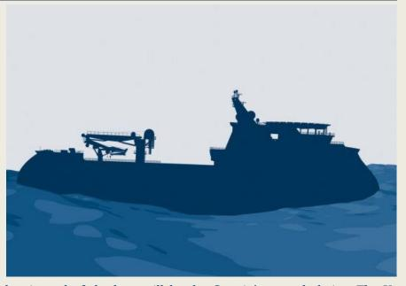
STERN<sup>TM</sup> towards the weather instead of the bow will be the Captain's natural choice. The X-STERN<sup>TM</sup> leads to reduced pitch and wave drift forces, as well as eliminating slamming. Positive effects are reduced power and fuel consumption while on DP, or the possibility of operating in a
