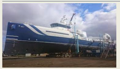
EVO partners, Diverse Projects (as owners representatives) and Oceania Marine Shipyards have been selected by vessel owners for this major project. The 51.30m **Umbra** is the second Sea Axe vessel built by the Dutch Damen Shipyards Group and has been slipped at Oceania Marine's North Shipyard in Port Whangarei, New Zealand for major upgrades. The aptly named vessel was launched in
