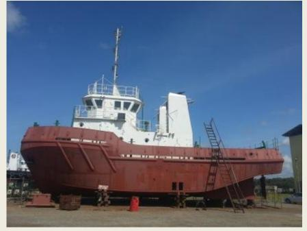
The Sibu, Sarawak based Rajan Maju Marine Industry yard continues to offer their successful handy size tug available on prompt delivery. The 23.5 by 7.315meter tug has a single chine 3.048-meter-deep hull. The keel is fabricated from 12 milometer steel plate while the bottom, sides and deck are all nine mm. Propulsion power is provided by a pair of Cummins KTA19-M3 Tier Π diesels each producing 447 kW (600 HP) at 1800 RPM. The
