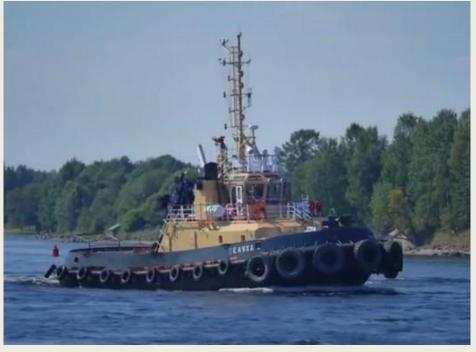
within the Baltic Fleet Navy. Assignment: The tugboat is intended for towing and berthing operations in harbor and coastal areas which comply with R2 navigation area (not more than 100 miles from place of shelter), performing of escort operations at the speed of 10 knots, refloating of ships and vessels, firefighting operations at floating and shore objects, oil and petroleum content products, cargo transportation, ice breaking and rescue and special purpose operations as well.
