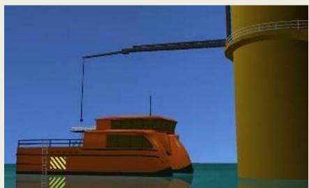
initiated by the UK Carbon Trust to encourage and discover innovative new ideas to accelerate the development of the offshore wind industry. As offshore wind farms move further offshore and in order to compensate for the number of non-productive bad weather days, TMD is re-engineering the 20m North Sea-Cat to provide two more production models. The first is a 35m x 12m North Sea
