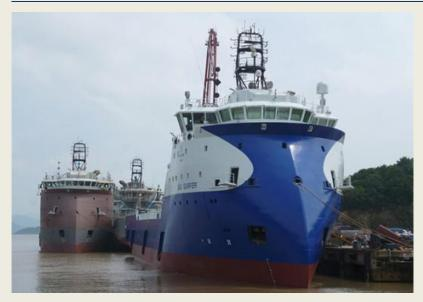
'Sea Surfer', the 10th of twelve platform supply vessels designed by Ulstein for Seatankers/Deep Sea Supply, was delivered from Zhejiang, China, on 18 July 2014. All twelve vessels carry the PX105 design. The vessels are 88.9 metres long and 19 metres in the beam and equipped with a diesel-electric propulsion system. The cargo deck area is approximately 1,000 m2 and the vessels each have a dead weight of 4,500 tonnes. The deliveries from Ulstein also
