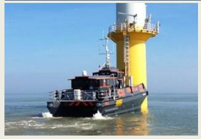
CTruk's third 20m SWATH (small waterplane area twin hull) is nearing completion and the company is currently organising demos of this innovative advanced FRP composite vessel before she leaves for an imminent contract with leading offshore solutions provider CWind. As you may be aware CTruk's second SWATH, CWind Endurance, has been working since delivery as a crew transfer vessel supporting cable pull in work on Westermost
