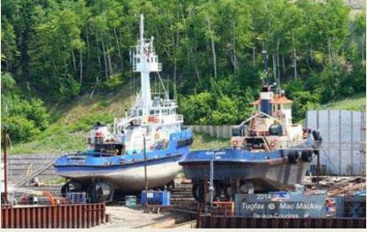
bilges of the fully molded hull of **Océan Echo II** versus the hard chine hull of Océan Basque. Neither tug has bilge keels to allow for working in ice. **Océan Echo II** has been replaced in wood chip barge service by **Mega** *+ Motti*, so is likely in for a long stay at the ship yard. Just visible at the bow is one of the hydraulic rams for barge connection. *(Source: Mac Mackay – Tugfax)*
