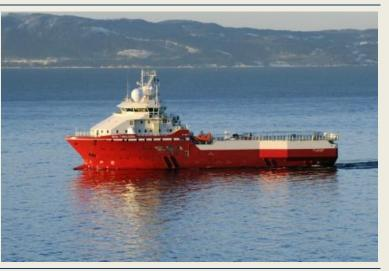
with a beam of 16,40m. Deadweight is approx. 3000 tonne and maximum speed is approx. 17 knots. The vessel is designed with dedicated working deck area arranged on 4 deck levels, accommodation is for 57 persons and a helideck aft for Sikorsky S-92 class. *(Source: Offshore Energy Today)*
