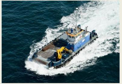
А geotechnical ground investigation is taking place at the proposed Burbo Bank 2 (extension) wind farm this month. 22meter multi The cat 'Willendeavour' will conduct a series of shallow vibrocore holes and cone penetration tests (cpts) at selected positions in the proposed wind farm footprint as well as along the proposed export cable route. Weather permitting, the operation is expected to run until mid-august. The extension project
