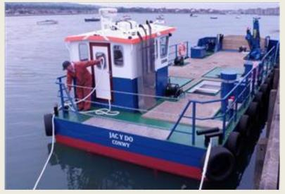
The latest Meercat has been launched for Conwy Harbour Authority, for use as a port service vessel. The monohull vessel **Jac Y Do** measures 14 x 5 meters and is powered by twin Doosan L136 sixcylinder heavy duty engines each developing 160bhp / 118kW at 2,200rpm, supplied by WaterMota. The vessel has been built to serve several uses including general harbor maintenance, doubling as a fully operational dispersal dredger while also being suitable for
