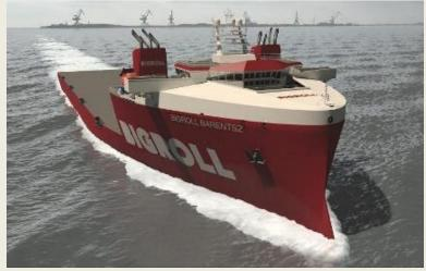
completely flush and open stern, with an open space measuring 42 m x 125 m. (Source: BigRoll)
