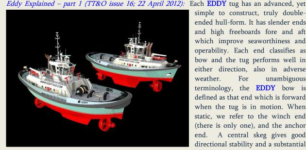
simple to construct, truly doubleended hull-form. It has slender ends and high freeboards fore and aft which improve seaworthiness and operability. Each end classifies as bow and the tug performs well in either direction, also in adverse weather. For unambiguous terminology, the EDDY bow is defined as that end which is forward when the tug is in motion. When static, we refer to the winch end (there is only one), and the anchor A central skeg gives good directional stability and a substantial
