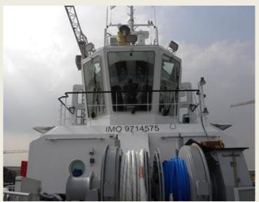
The front view of the wheelhouse. The wheelhouse has a split level design, providing excellent allround visibility. The forward control station, of typical split parallel console type, afford the helmsman maximum visibility to both fore and aft deck working areas.
