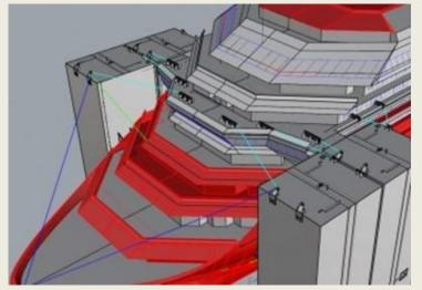
Installation of sponson S7 on the starboard side of the **Concordia** wreck has been completed, the salvage team said on Sunday, May 25th. This is the sixth out of a total of 15 refloating sponsons that will be attached to the starboard side of the wreck. In addition, Barge Micourier2 is at the site carrying sponsons S6 and S5 on board, pending installation of S6 which is about to ensue. Once the installation of all sponsons is completed, a pneumatic system will be used to empty the water
