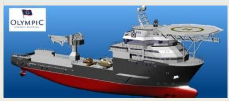
Kleven has signed a contract with Olympic Shipping for the building of an MT 6021 MKII design IMR vessel. The contract value is around NOK 450 million (USD 75.5m), and the vessel will be delivered from Kleven Verft in June
