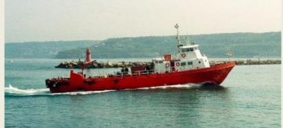
overall: 30.42m a draft (max): 1.6 m a grt of 114 tons and a nrt of 34 tons. They have three General Motors 12V92 TA main engine with a total output of 2,495 hp. The vessles have a Clear Deck Space of 50m2 and an accommodation 40 and 50 pax capacity respectively for each boat. *(Source: Arena Offshore Brokers)*
