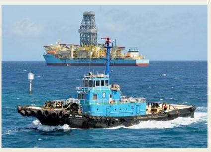
has a length o.a. of 36,26 mtra a beam of 10 mtrs a depth of 4.44 mtrs a grt of 368 tons a nrt of 110 tons and a dwt of 199 tons. The two Niigata 6L28HX main engines develops a total output of 2.650 kW (3.600 hp). She has a free sailing speed of 14.2 knots and a bollard pull of 43 knots. She is classed Bureau Veritas. *(Photo: Kees Bustraan)*
