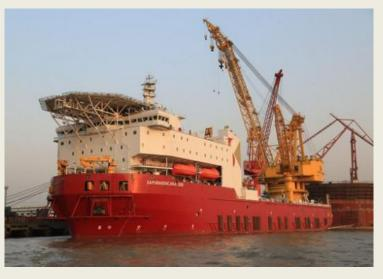
positioning system, which enables it to carry out heavy-lifting installation of large-scale offshore structures such as platform blocks, modules and jackets, as well as S-type pipe laying operations in water depths of up to 1,500 meters. The vessel measures 156.4 meters in LOA (length of all), 44.8 meters in breadth, 16.8 meters in depth, with a design draft of 7.4 meters and a lifting capacity of 3,500 tonnes. *(Source: World Maritime News)*
