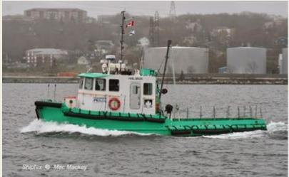
Basin. Built in 1960 by and for Halifax Shipyards, it was completely rebuilt in 2009 by current owners Dominion Diving. At that time it was repowered with an 8V71 main engine of 318 bhp and given a 12 inch bow thruster. *(Source: Shipfax@Mac Mackay)*
