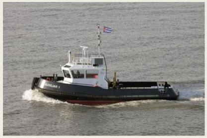
output of 894 bkW (1.216 bhp). She achieved 16.6 ton bollard pull and a speed of 11,2 knots. The tug is classed Bureau Veritas I HULL • MACH Tug Coastal Area. *(Source: Damen)*
