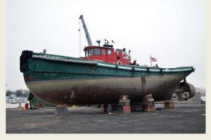
The Great Lakes Towing Company begins work on Tug Wyoming as part of its ongoing fleet overhaul program. Drydocking routine and maintenance for Wyoming includes: • Typical US Coast Guard Inspections; • Drydocking and Routine Maintenance and Repairs; • Blasting and Painting; • And Other Various Cleaning, Inspections, and Repairs; The 17 tons bollard pull tug is the 10th tug to be overhauled and
