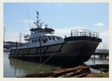
Seacat Services, offshore energy support vessel operator, launched its latest 24-metre British-built South Catamaran, named Seacat Ranger. For the launch of Seacat Ranger, the latest 24-metre DNV GL class-certified vessel to be built in the UK, incremental build improvements include a new bow and fender design that enhances stability when the vessel is pushing onto the wind turbine foundation. Further modifications include additional crew loading and access space near the bow, to help
