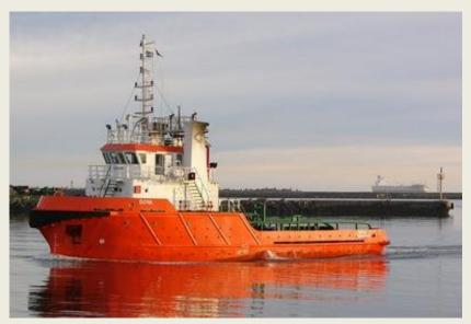
sign 9V2271 Offshore Tug Supply Vessel Subject Dova (Imo 9714317) to uplift bunkers. The tug is owned by International Bulk Trade Pte. Ltd. - Singapore and managed by SMC Marine Management Pte. Ltd. – Singapore. She has a length o.a. of 31.65 mtrs a beam of 9.14 mtrs and a depth of 4.20 mtrs. The grt is 295 tons and dwt 270 tons. The Dova is built by Hung Seng Shipbuilding Sdn. Bhd. – Sibu; Sarawak; Malaysia
