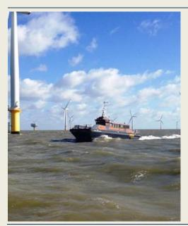
next generation CWhisper SWATH 20m workboat, **CWind Endurance**, is currently working out of the ABP Port of Grimsby. A third is currently in production at CTruk's Brightlingsea base. The SWATH hull form (SWATH stands for small waterplane area twin hull) gives a smoother ride in rough seas, vastly improving comfort levels for technicians commuting to offshore wind farms in rough conditions. To know more visit www.ctruk.com/products-and-systems/cwhisper (*Press Release Ctruk*)
