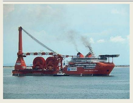
The Lewek Constellation, the latest addition and flag ship of Emas. The new vessel will have an overall length of 178.27m, moulded breadth of 46m, moulded depth of 15.6m and maximum draft of 10.5m. Its net tonnage capacity will be 14,636t and gross tonnage capacity will be 48,786t. The vessel will have a deck area of 4,200m<sup>2</sup> minus the reels and possess deck strength of 10t per m2. It will be equipped with a K-POS (Kongsberg Maritime) DP3 system integrated with
