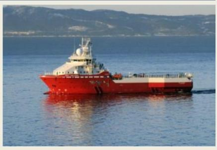
used for the operation. The vessel of the MT 6007 design is one of the world's first custom built-ships for seabed logging operations to detect hydrocarbons beneath the seabed. The ship's length overall is 80,35 m with a beam of 16,40m. (Source: Offshore Energy Today)
