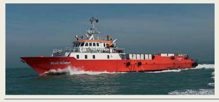
**'Blue Mommy'** Constructed at the Vittoria shipyard in Adria, the all-aluminium FSIV **'Blue Mommy**' has a length of 56 metres, a speed of 28 knots and a capacity of 71 passengers and 140 tonnes of cargo. Upon delivery, the vessel has headed to West Africa for offshore operations. She is rated for DP-2 dynamic positioning and features a mixed propulsion system of both propellers and waterjets.
