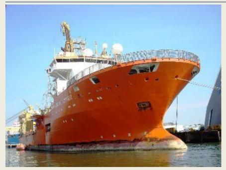
Multi-Purpose Offshore Vessel 'Normand Cutter' has arrived at Damen Shiprepair Rotterdam for repair and modification work. The 127, 5 m long deepwater subsea construction and umbilical lay DP vessel has been drydocked at the repair and conversion yard, Damen through social informed media. The scope of work the vessel includes: on overhaul of all four main engines, overhaul of the 300-ton SWL National Oilwell offshore crane, hull
