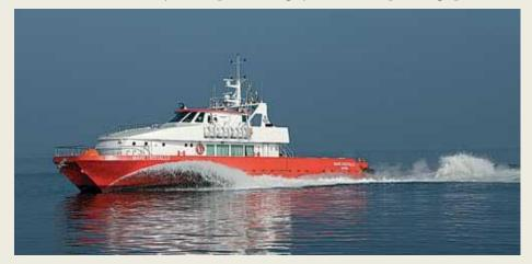
'Mare Cristallo' The aluminium crew boat 'Mare Cristalo' measures 30 metres in length with a capacity of 45 passengers and 30 tonnes of cargo. Featuring special purpose ship classification, the vessel's cruising speed is 20 knots.
