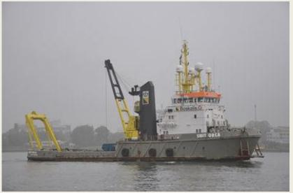
Unie van Redding & Sleepdienst – Antwerp; Belgium. The vessel has a length o.a. of 50.70 mtrs a beam of 11.50 mtrs and a depth of 4.70 mtrs. The two main engines develops a total outpu of 1,400 kW. She has a speed of 10 knots and a bollard pull of 30 tons and is classed Bureau Veritas. *(Photo: R&F van der Hoek-Lekko)*
