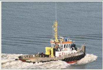
develops a total output of 1,492 kW (2,028 hp) and a speed of 10 knots. She is classed Bureau Veritas nr. 08322X with notations I 🔮 Hull • Mach Tug Unrestricted navigation AUT-UMS, ICE CLASS ID. *(Photo: Reinier van de Wetering)*
