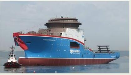
to join Marine Platforms' fleet. The 113-metre long multipurpose service vessel is going to sail under the Nigerian flag into the country's waters in September. It has a gross tonnage of 5000t and its main crane is 3000-metre long. *(Source: World Maritime News)*
