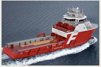
Vard Langsten has delivered AHTS Far Sirius (UT 731 CD) to Farstad Supply AS, a wholly owned subsidiary of Farstad Shipping ASA. The UT 731 CD vessel is designed to work in extreme environmental conditions and carrv out operations in waters as deep as 3,000 metres. With a total length of 87.4m, breadth of 21.0m, the ship has a bollard pull of approx. 260 tons and installed power of approx.
