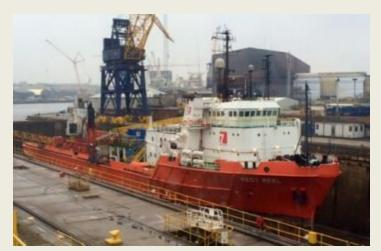
site in Tyneside bringing the 'DP Reel' Offshore Support Vessel. The 90 x 18m vessel required inspection and specialist repairs to the Forward Azimuth Thruster. Other works included Port & Starboard Tailshaft seal renewal. removal of temporary deck equipment from last charter, modifications to the automatic sprinkler system, removal and refurbishment of Main & Auxiliary Engine Fuel Pumps & Governors by specialists, resetting of fuel timing and modifications to existing TLQ's steel
