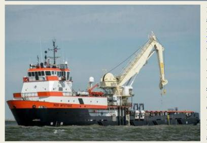
Harkand has entered into a charter agreement with Hornbeck Offshore for the offshore construction vessel HOS Mystique for a firm period of two years plus options. The 250ft (76.2m) DP2 vessel has a 70 MT AHC crane and will be outfitted with a Harkand Triton XLS ROV to support IRM and survey work in water depths up to 3,000m in the Gulf of Mexico. AJ Jain, North America managing director for Harkand said: "This strategic addition to our growing fleet gives
