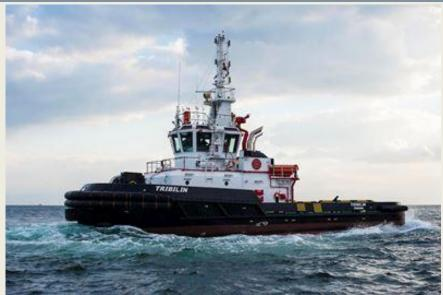
breadth moulded is 11.70 m and has 2 x Caterpillar 3516 C, total 4200 kW main engine and Schottel SRP 1515 CP Azimuth propulsion system. *(see Tugs Towing 7 Offshore Newsletter issue nr. 18 also).* Her is seen the tug during her technical trails in the Marmara Sea. *(Source & Photo: Bogazici)*
