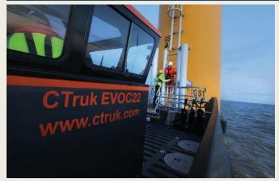
22m multi-role composite cat will have 24,000 litre fuel capacity. Whilst debate continues about the most efficient way to serve offshore wind installations further out to sea, CTruk has been quietly forging ahead with a new OWSV designed to safely deal with rougher seas, longer transits and tougher assignments whilst not neglecting the comfort of passengers and crew. Based on a proven workboat design concept,
