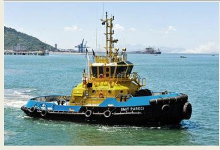
Keppel Singmarine Brasil Ltda. (KSMB), of Navegantes, Brazil have completed recently the construction of the SMIT **Pareci**, the second of a series of six Robert Allan designed RAmparts 2500 tugs, for SMIT Rebocadores do Brasil (Rebras), of Rio de Janeiro. The **SMIT** Pareci was delivered in December of 2013, and follows its sister, the **SMIT Pataxó**, which was delivered in June of 2013.
