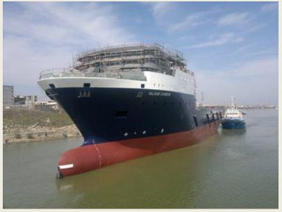
area of approximately 650 sq.m. According to Rolls-Royce, the UT 755 is one of the most popular PSVs ever constructed, and more than 200 vessels of this model have been built or are under construction. The CD version is delivered with a diesel electric machinery system and Azipull or US thrusters or as a diesel mechanic version with conventional shaftlines. *(Source: Offshore Energy Today)*
