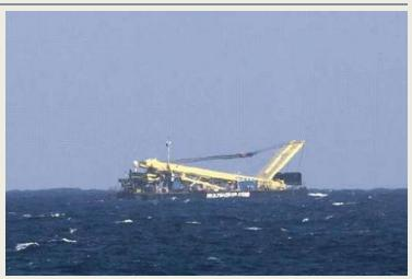
*Photo EPA). Sheerleg:* The transport turned out to be a sheerleg vessel, named **Cormorant**, of Multraship from Terneuzen. Eline Muller of the company says to Omroep Zeeland that the transport is on its way to Nigeria. The sheerleg will be deployed in the wreck removal in this African country. Due to the fact that the legs are down the sheerleg look different than normal. It is certainly conceivable that the ship, according to Eline Muller seen from afar looks as an airplane.
