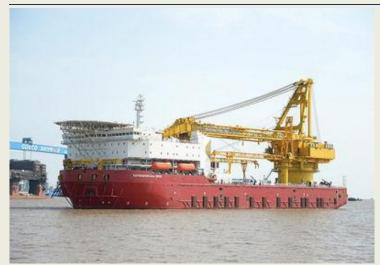
COSCO Nantong shipyard has delivered a pipelay heavy lift vessel, 'SapuraKencana **1200**′ to SapuraKencana Petroleum, Malaysia's premier integrated oil & gas services solutions provider. and The SapuraKencana 1200, developed by Ulstein Sea of Solutions, is designed as a self-propelled vessel with a 10-point mooring system for operations in water depths up to 200 meters. Classed by ABS, the ship is also equipped with a DP3 dynamic
