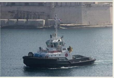
30.25 mtrs a beam of 11.75 mtrs and a draught of 3.75 mtrs with a grt of 463 tons and a nrt of 139 tons. The two Caterpillar main engines develops a total output of 4,000 kW (5,434 hp). She has a speed of 12 knots and is classed I Hull Mach Tug-Firefighting ship 1 -water spraying Unrestricted navigation. *(photo: Capt. Lawrence Dalli - www.maltashipphotos.com)*
