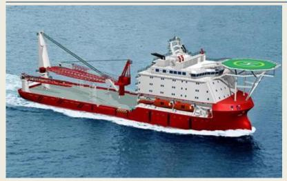
Focal Marine & Offshore, a Singapore/Shanghai based OSV designer, has won a design contract for a DP-3 Offshore Construction Vessel (OCV) from one of their regular clients. **FOCAL 530 design** has a high DP capability, which is achieved by five thrusters, enabling the design to be suitable for operation in deep waters of the Gulf of Mexico, Brazil, West Africa etc. The other pieces of
