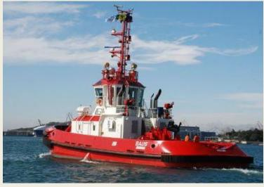
compartments. On main deck there are single cabins for captain and chief engineer and amongst other changes from the slightly less beamy version is an entirely separate galley and mess room arrangement. Other changes earlier and improvements over versions include a full FiFi1 external fire-fighting system, Karmoy hydraulic winches fore and aft driven via main engine PTO and increased wheelhouse foot print with access both sides. Sanmar also claims that a new skeg design has benefited the
