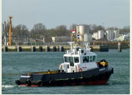
Last Wednesday March 19, 2014 was seen on the Caland Canal in the Rotterdam Europoort near the Heerema location the Damen new building StanTug 1907 with yard number 503419. The commence technical tug trails and bollard pull tests. The standard tug has a length of 19.34 mtrs a beam of 7.34 mtrs and a depth of 3.39 mtrs. The total engine output is 1,492 bkW with a bollard pull of 27 tonnes and a speed of 11.7 knots. (Photo:
