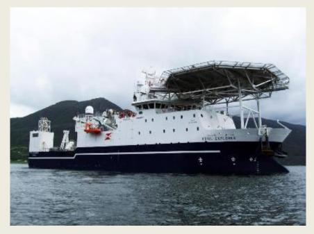
MMT has signed a long term charter contract for M/V Stril Explorer that is operated by Simon Mökster Shipping AS. MMT has during several projects in the conducted various past survey assignments from this vessel. M/V Stril Explorer is a DP2 offshore vessel with a large open deck and is very suitable for launch and recovery operations, for example with ROVs, AUV and geotechnical equipment. The vessel is equipped with a 60 T offshore crane with a
