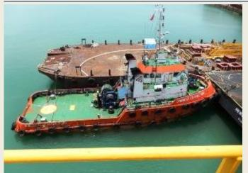
**Swiber Charlton** seen from the Derrick barge *Swiber Triumphant* at the NSE Yard in Singapore. The tug has a length o.a. of 33.00 mtrs a breadth moulded of 9,76 mtrs and a depth moulded of 4.30 mtrs. She has two Cummins KTA50 diesel engines with a total output of 3,200 hp at 1,800 rpm. A speed of 12 knots and a bollard pull of 40 tons. The tug is classed Bureau Veritas. *(Source: Ger Maijntz)*
