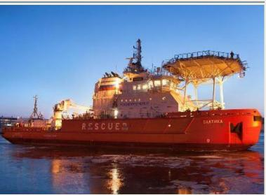
River Transport in spring 2014. The vessel will be used in icebreaking, rescue and oil combatting operations in the Gulf of Finland. *(Source: Arctech)*
