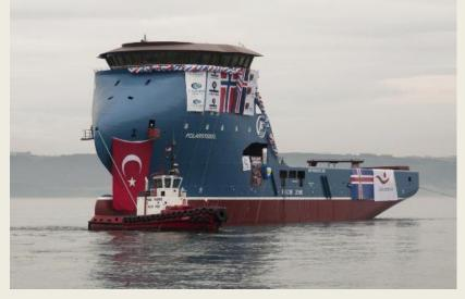
Cemre Shipyard launched a new ship built for Norwegian Havyard Group based on the order of Icelandic oil service company Fafnir Offshore on 1 March 2014. The vessel, **Polarsyssel**, is a state-of-theart platform supply vessel (PSV) of Havyard 832L L WE design, specially built for operations under extremely harsh conditions in the North Atlantic. She is 88.5 meters long and 17.6 meters wide.
