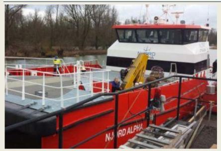
Njord Offshore is about to add a 26m Damen 2610 Twin Axe Crew Transfer Vessel. the Njord Alpha to the fleet. Njord Offshore has worked with Damen to create an optimised vessel to suit its needs, making minor changes to the standard design to improve comfort, efficiency and safety. The vessel is designed and classed to BV Classification I X Hull MACH Light Ships/Fast Utility Vessel standards. The
