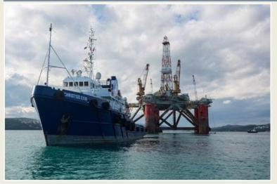
Panama Registered OSV / AHTS Christos XXIII, 8000 bhp, 95 tbp, operated by Spanopoulos Group S.A was successfully handled another one demanding rig move / towage operation. OSV / AHTS Christos **XXIII**, as Lead tug has safely delivered her tow Semi submergible Rig Pentagon 91 Type Zagreb 1 (Length 103.4 mtrs / Breadth 106.3 mtrs) from the Shipyard of Brodotrogir in Croatia towards delivery handover point /
