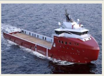
SERIES comprises a wide range of platform supply vessels designed by Vard Design in Ålesund, Norway. The PSVs are designed with high focus on cargo capacity and excellent maneuvering capabilities combined with low fuel consumption. (Source: VARD)
