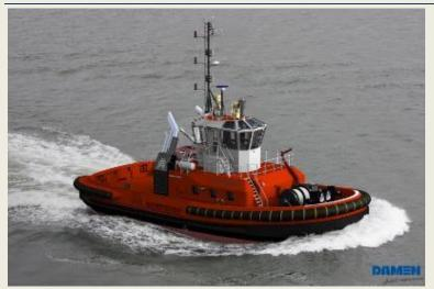
operator Leading Italian tug Rimorchiatori Riuniti has ordered a powerful Damen ASD Tug 2411. Reflecting the industry's move to larger vessels, the new Damen tug, which has a 70-tonne bollard pull will replace a smaller 1990-built, 40-tonne unit. The new vessel will be deployed in Genoa and is expected to arrive by end-July. Owned by the Delle Piane and Gavarone families, Rimorchiatori Riuniti has been operating its well-
