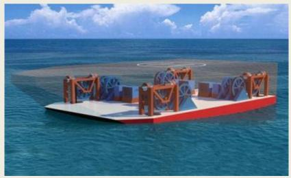
also combines both the wave generators and the current generator frames. The advantage of this system is that most of the components are located above the water, allowing easy access for regular maintenance and efficient major equipment replacement offshore. Being a low profile structure, the barge does not make a significant visual impact, and is invisible when over 10 miles offshore. (Source: Offshore Wind)
