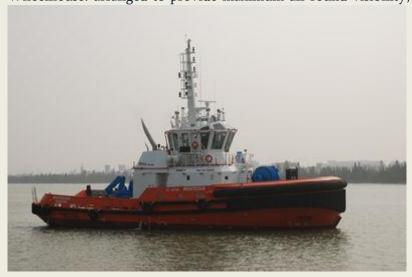
and a split console forward. A chart table is located to port. Main Deck: • Deck machinery: Forward hawser winch/anchor windlass; Aft towing winch and gob eye; deck crane and tugger winch on aft deck; mooring bitts forward, midship and aft. • Mess / Lounge / Galley: comfortable seating area with television and an area for the crew to enjoy a meal between shifts. • Flushmounted, machinery access/ flush removal hatch.
