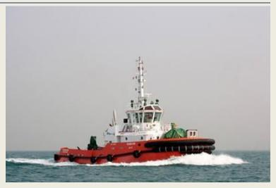
exceptionally well-proven ASD tug designs. Each of these designs has been developed from a successful prototype vessel or series of vessels, and refined to emphasize ease of construction. Each new delivery is also custom-tailored to the needs of each individual Client. Robert Allan Ltd. worked closely with Cheoy Lee Shipyards and Yuexin Ocean Engineering Co. Ltd in the design
