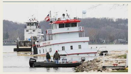
Investigators found out the the "Stephen L. Colby" which sank in the Mississippi River at LeClaire was damaged when it struck a rock on Nov 25, 2013. The tug got close to shore before it sank in shallow water. An eight-mile stretch of the river was closed as crews cleaned up thousands of gallons of diesel fuel spilled into the water. The gashes in
