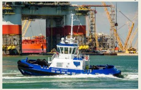
stern winch is primarily used for tie-up work and light tows. Two John Deere 60-Hz, 480-V generators provide 125 kW each. On the bridge deck is remotely operated, 1,000-gpm, Akron Brass 3678 fire monitor powered by an AMPCO ZCH pump with a Baldor electric motor. Signet Maritime collaborated with Robert Allan Ltd. on eight ASD
