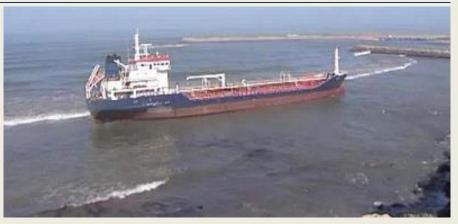
iron wires. The pumping rate was 65 tons per hour. The oil was transferred to the thermal station of Tan-Tan, 1.5 km from the accident site, and stored in a tank with a capacity of 5000 tonnes. The operation involved 182 tank trucks with a capacity of 25 tons each. Regarding the salvage, a tug with a power of 3,000 hp was coming from Casablanca and expected on scene at midnight. (*Photo: Le360Live*)
