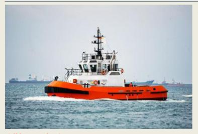
Arena Offshore Brokers Ltd.-Istanbul is pleased to announce the delivery of a 2013 built -Shallow Draft Harbour Tug, to the Nigerian clients. The 2013 Turkey built Shallow Draft Harbour Tug has a length o.a of 19.95 mtrs a breadth of 7.00 mtrs and a draft of 2.20 mtrs. The two CAterpillat main engines develops a total output of 1,200 bhp 1,800 rpm. The bollard pull of the tug is 15 tons. There is accommodation for 6 person. She is classed RINA. (Source: Arena
