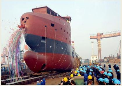
Zhenjiang Shipyard held, on January 3rd 2014, a launching ceremony for the first of six supply all-electric platform vessels of VARD PSV08 design, which are being built for Tidewater Co., Ltd. Having the length of 83.8 meters, breadth (MLD) of 18m, depth (MLD) of 8.4m, the PSV boasts of carrying capacity of 4100t and 870 m<sup>2</sup> of deck area. The vessel is equipped with an advanced Blue™ Drive Plus C power-supply system. Based on
