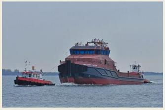
beam of 4.20 mtrs and a depth of 1.80 mtrs. The GM Detroit diesel type 12V71N develops an output of 268 kW (365 hp). She has a bollard pull of 5 tons. The sistership **Vliestroom** built in 1969 has the same specifications as the **Merwestroom** the only difference is the raised wheelhouse for pushing purposes. (Source: van Wijngaarden; Photo Huib Trommel©)
