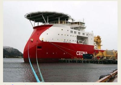
Ceona's high-capacity flexible/umbilical pipelay and subsea construction vessel, the Polar Onyx, has been floated out of dry dock at Ulstein Verft yard in Norway following an intensive outfitting programme. It has now moved to the shipyard quay where the interior works will be completed and the systems brought online. Designed to the highest standard for dynamic positioning, DP-3, the vessel is equipped with a 250t AHC offshore crane. Like Ceona's flagship vessel,
