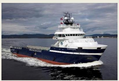
said, "This is our 20 vessel built at Vard Brevik, with four more yet to be delivered." The vessel has an overall length of 84.45 meters and a breadth of 17 meters with a deadweight of 3,800 metric tons and a deck capacity of 800m2. M/V Island Duchess will be transporting pipes and general deck load, liquid cargo as well as cement and barite to drilling rigs in the North Sea. She is also prepared for later duties as standby/rescue
