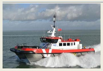
We are pleased to announce that MPI Workboats has taken delivery of MPI Altisidora on 22 October 2013. MPI Altisidora is a windfarm-support vessel, built at the South Boats shipyard on the Isle of Wight. She is the ninth addition to the MPI Workboats fleet. Vessel particulars: Length overall 19.15 m; Beam overall 7.25 m; Draft 1.20 m; Tonnage 40 tonnes; Total fuel capacity 6,000 ltr; Endurance 350 nm (15 hrs @ 22 knots); Water capacity 200 ltr; Passenger facilities
