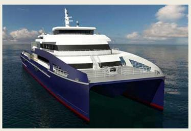
multiple offshore workers to installations, with the hull design optimised for high-speed transits with noise, vibration and climate control features limiting the seasickness of transiting offshore workers. The vessel is also designed to operate in sea conditions of 40-knot winds and three-metre seas. Four MTU 16V4000 engines will power the vessel, driving HamiltonJet HT-900 water jets to a service speed of 30 knots fully loaded. Four azimuthing drop-down thrusters
