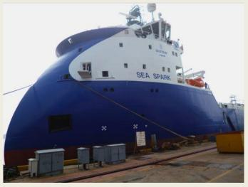
BOW® hull line design. These vessels have low vibration levels, resulting in increased comfort, and no speed loss due to the elimination of bow wave impact. The vessels can maintain higher speed even in foul weather, and the operational window is increased. (Source: Ulstein)
