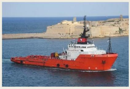
of 15.91 mtrs and a draft of 6,89 mtrs. The two MaK 8M35 develops a total output of 10,900 bhp. The speed is 16 knots and the bollard pull 140 tons. She has a grt of 2,311 tons and a dwt of 2,499 tons and is classed Det Norske Veritas. *(Photo: Capt. Lawrence Dalli - www.maltashipphotos.com)*
