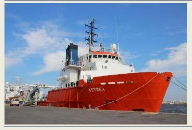
Operating from Den Helder (photo) and IJmuiden and chartered by the Dutch diving company N-Sea the Greek survey vessel **Astrea** is working in the offshore industry. The 71-metre long vessel, fitted out with an A-frame, installed concrete mattresses on a new pipeline in the Dutch sector of the continental shelf. *(Source & photo Paul Schaap)*
