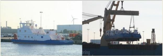
In the past week two pusher tug were loaded on the heavy cargo vessel BBC Amethyst. The pusher tugs **Impala Puerto Wilches** and **Impala Zambrano** were built by Shipyard "De Kaap" – Meppel; Netherlands and loaded in the Westhaven - Amsterdam by the BBC Amethyst own equipment. The pusher are bound Barranquilla – Colombia. *(Photo: Hans Windhorst)*
