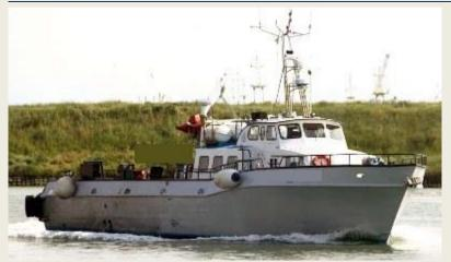
Blue Sea Brokers confirm they have now sold a Supply Crew Boat from Italy to Spain. The vessel is a 30 m twin screw supply crew boat with total power 1268 kW. It is Classed with RINA and has capacity for more than 30 passengers - personnel and a free deck space for cargo as well as certificates for carrying dangerous goods. *(Source and photo : Blue Sea Brokers*)
