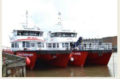
Alicat have launched their second next generation vessel following the launch of the 22m DNV Class Dalby Aire in the summer. This 19m vessel, named **Solway Challenger**, is powered by two MAN V12 engines and Rolls Royce water jets. Emphasis has again been made on greater foredeck working space and both vessels can comfortably carry a 10ft container on the foredeck with a cargo weight of 7.5T and 5T respectively. *(Source: Alicat)*
