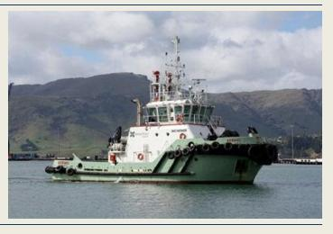
Timaru Ltd – Timaru; New Zealand. She has a length of 28.00 mtrs a beam of 9.80 mtrs and a depth of 4.90 mtrs. Her grt is 318 tons and the nrt 95 tons. The two Yanmar type 8N21A-EN main engines develops a total output of 2,648 kW (3,600 bhp) at @900 rpm. Her speed is 12 knots and bollard pull 50 tons. The tug is classed Lloyd Register of Shipping. *(Photo: Alan Calvert)*
