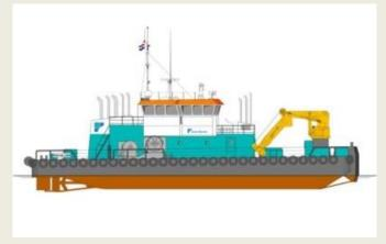
Leading workboat operator Acta Marine is further expanding their fleet with a new multipurpose workboat with Dynamic Positioning and more than 35 tons bollard pull. The vessel, which will be named "Coastal Chariot", is a sister vessel of Acta Marine's existing DP-1 unit "Coastal Challenger". The multipurpose vessel has the following main characteristics: • 35 by 12 meters; • Propulsion power: 2,380 Kw (2 x fixed pitch propeller in nozzle and 1
