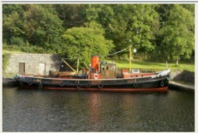
The Duke of Normandy II seen at the basin of the Crinan Canal, Crinan, where she has been based for the last few years. [54grt 70.9 x 14.4 x 5.8 ft. 350bhp (re engined 1958 with the installation of new Mirrlees 290bhp engine.)]. Built in Germany in 1934 as a river customs vessel she was requisitioned by the Kriegsmarine during the Second World War, as a Harbour Protection Vessel. under the designation FK01.
