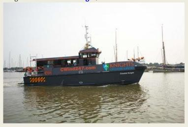
to meet the complex demands of the offshore wind support sector, the 20T MPC comfortably accommodates 12 technicians for transfer in its crew pod and can also reconfigure to carry a substantial payload on fore and aft decks of 37m<sup>2</sup> and 34m<sup>2</sup>respectively. managing director Ben Simpson said 'We are delighted to deliver Coastal Knight and wish Knights Offshore Support every success. Paul's belief in the merits of our innovative product
